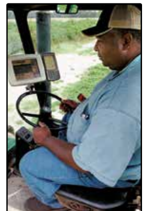
Figure 16 depicts a cab-mounted GPS and light-bar system. With this system, the skip and overlap
